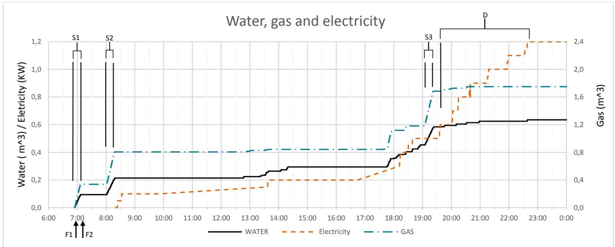
Fig. 7. Water, gas and electricity meter reads.
